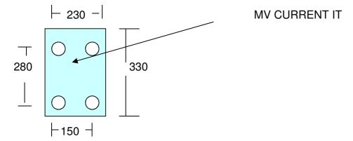
Dimensions are understood from the centre of each hole (in mm) Hole diameter is 15mm; oval shaped holes are 15x80 mm
